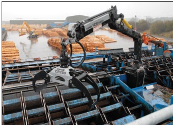
Static Mounted Crane on Sawmill Log Line
