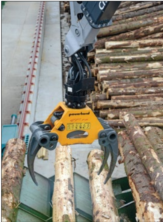
Well Protected Hydraulic Cylinder & Hoses
